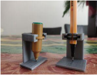
Vertical alignment rig with 'real' pen (left) and custom pen holder (right)
