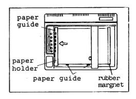
As a plotting paper, any high quality, coat on measuring paper can be used, but a coat paper due to its less blotting is suitable for this purpose. In addition, a film sheet for OHP (overhead projector) can be used. However, in this case use an oily pen.
