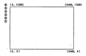
(2) Operation area and off-scale processing Even if the input applied as the parameters of commands AA,AR,CI,EA,ER,EW,FT,PA,PD,PU,PR,RA,RR, and WG exceeds the area of A3 size, 15400x11200 shown in the above figure, it becomes valid when it is in the operation area shown in the following figure. However in this case, the pen is off-scale-processed so that it does not move beyond the plotting area.
