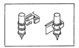
After any plotting will be finished, remove the pen from the pen stocker, and then insert it into the pen stand to prevent its tip from drying. When it is not used for a long time, store it with the pen cap covered.
