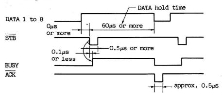
(6) Input connector (Interface conforming to Centronics)
