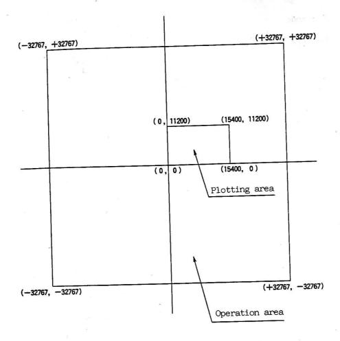
Note: Figures in parentheses show coordinates in steps of 0.025mm when the origin as a plotter is set to (0,0).
